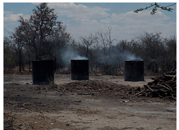
Photo taken during TFT field assessment. Smaller mobile kilns emit fumes that are dangerous to humans and nature alike. This way of preparing the charcoal also loses much of the potential energy of the wood, with 82% of wood energy lost before the product is burnt by the end-user. [5]
